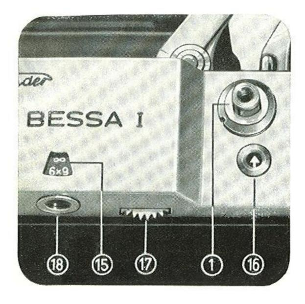
The optical finder can be adjusted for either of the two negative sizes of  $3^{1/4} \times 2^{1/4}$ " (6×9 cm) and  $2^{1/4} \times 1^{5/8}$ " (4.5 × 6 cm), as well as for near and distant subjects, to compensate parallax.
